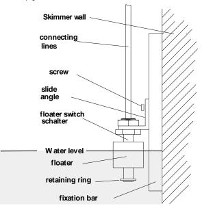
As part of the system maintenance, the mini liquid level switch should be checked regularly for damage and proper function.
