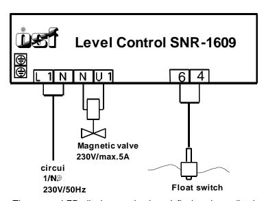
The electric cable of the float switch can be extended up to a length of 50m by use of a shielded cable (2x0.75mm²). The shielding is to be connected with clamp 4. Please note, that it is absolutely necessary to carry out the connections waterproof. The connecting cable of the float switch must not be wired together with other live wires.
